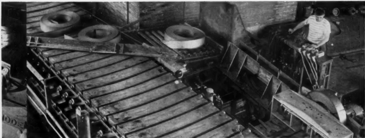
This MH10 push-button strapping machine has been strapping hot coils—1200° F.—dependably since 1953, at a rate of 120 coils per hour, 3 straps per coil.
